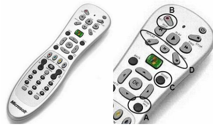
Figure 5: 9 buttons on the remote control were used. MORE INFO (A) toggled the visibility of the 'Related Videos' window in StaticList and DynamicList, REC (B) added a video to the queue, GUIDE (C) displayed the Guide, and '<' and '>' (D) navigated the queue.
